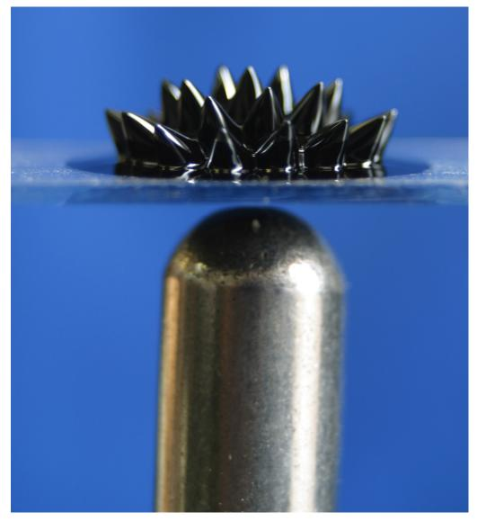
Adjust the power to the electromagnet to make the ferrofluid go up and down.
